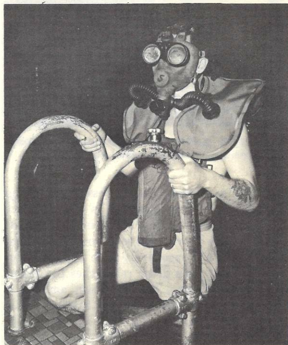
FIGURE 1-11.—Self-contained apparatus: closed-circuit scuba (Lambertsen amphibious respiratory unit "LARU").
