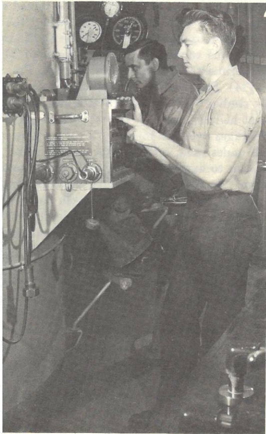
FIGURE 1-3.—Pressure tank, Experimental Diving Unit. The two wet-pressure tanks in the Deep Sea Diving School are used for training in deep diving; those in the Experimental Diving Unit are employed for the testing of decompression tables and for experimental dives.
