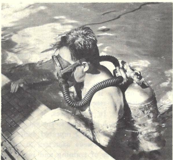
FIGURE 1-10.—Self-contained apparatus: open-circuit scuba.
